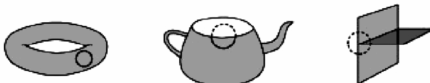
Figure 2. Manifold, manifold with boundary, and non-manifold surface, the picture is taken from [9].
