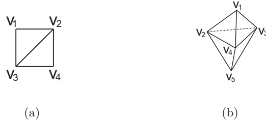
Figure 3.26: Each diamond is composed of two neighboring simplicial mesh cells, sharing a common face. Reference diamonds are depicted for 2D (a) and 3D (b) simulation mesh.
