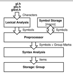
Figure 9.1: C Header file reader data flow scheme
